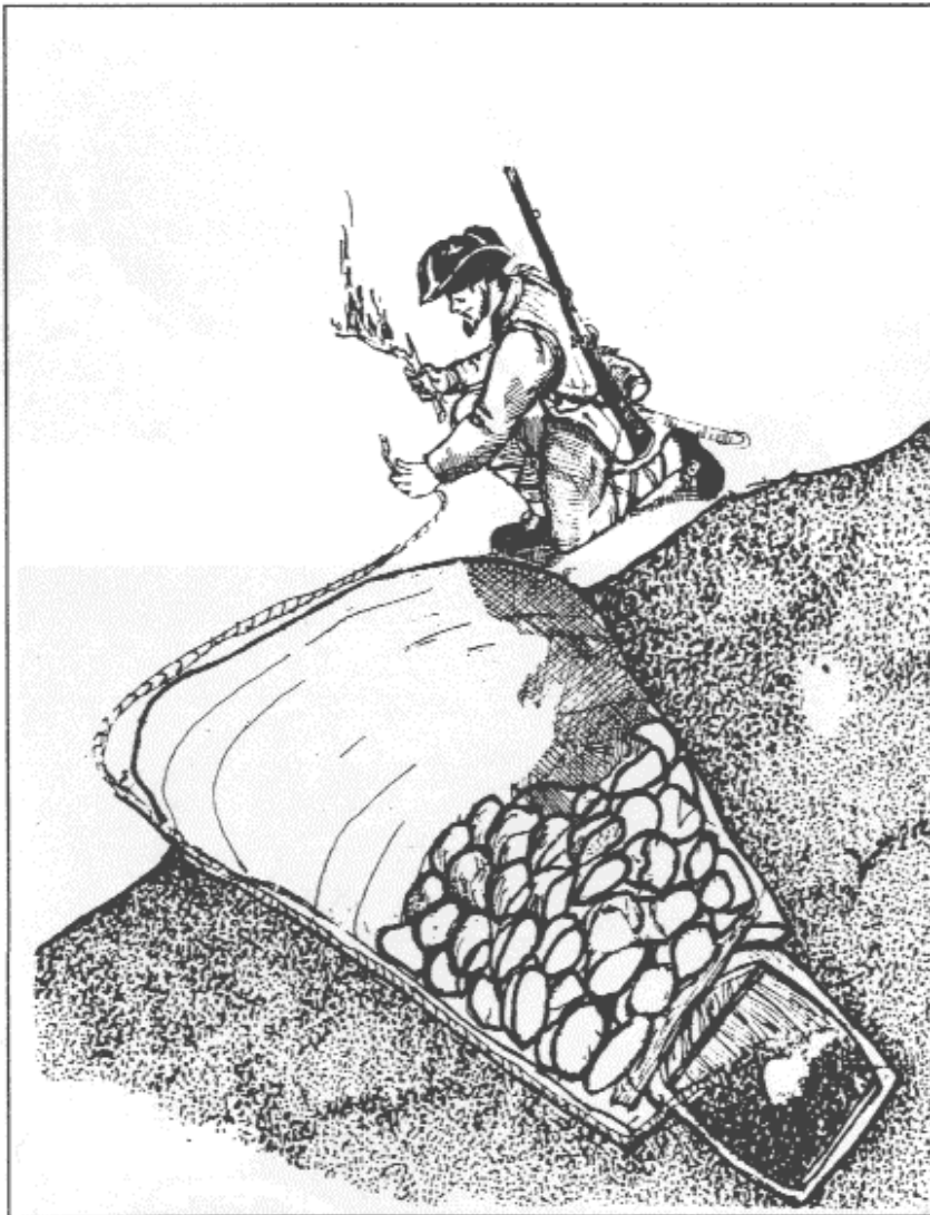
Above, section of a typical fougasse armed and ready to be fired. The militia trooper is about to light the long fuse cord that will burn its way down a narrow channel to the gunpowder barrel at the base of the fougasse. The resultant explosion would propel the mass of rocks to a distance of 300 ms.
